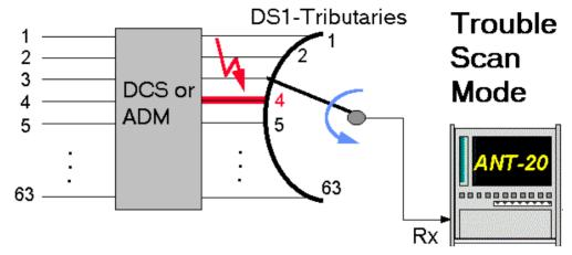
Fig. A-12 Alarm status recalled (Trouble Scan)
