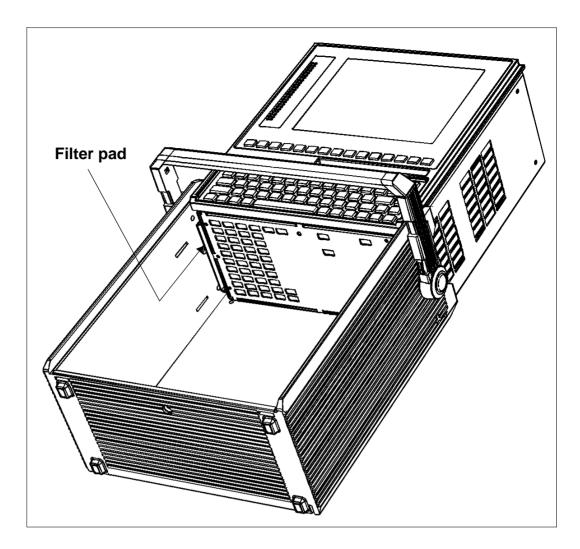
Fig. M-4 Replacing the ANT-20 filter pad
