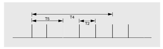
Fig. TB-6 Periodic pointers with one missing pointer, e.g.  $T4 = 5 \times T2$
