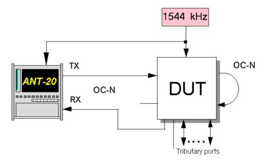
Fig. A-38 Pointer stress test setup
