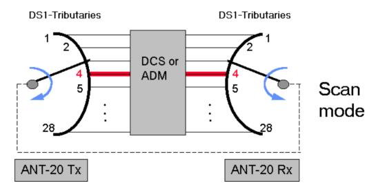
Fig. A-17 Automatic Scan mode
