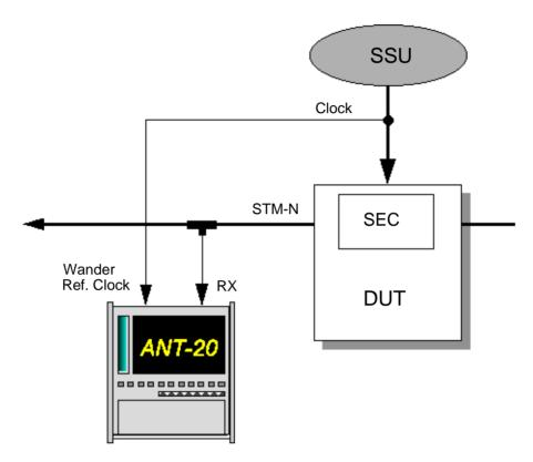
Fig. A-79 Wander measurements setup
