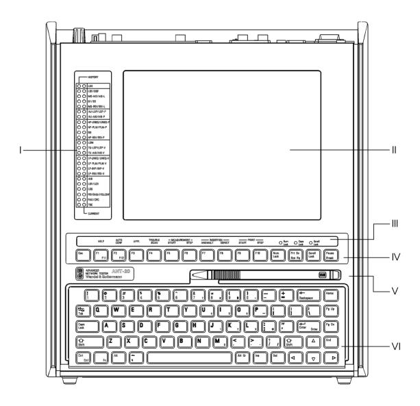
Fig. O-1 ANT-20, ANT-20E front panel
