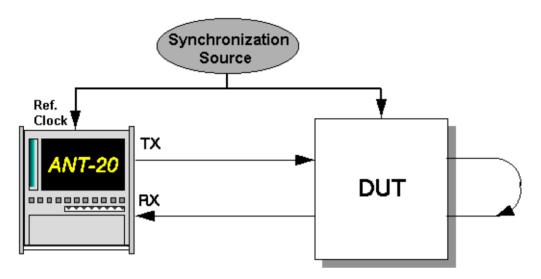
Fig. A-85 Test setup for measuring maximum tolerable wander
