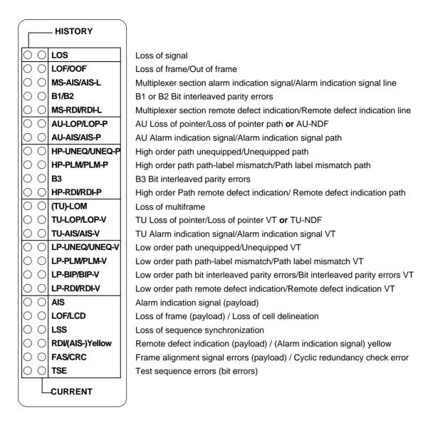
Fig. O-5 Meanings of the LED indicators on the ANT-20 front panel
