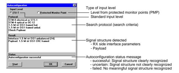
Fig. VI-5 "Autoconfiguration" dialog
