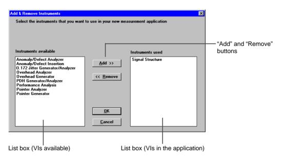
Fig. O-17 The "Add & Remove Instruments" dialog window of the Application Manager
