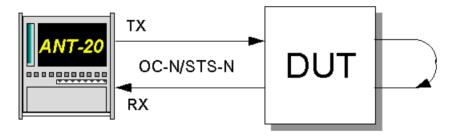
Fig. A-35 Out of service measurement setup
