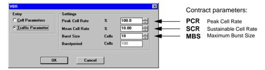
Fig. A-124 "VBR" dialog box in the "ATM Signal Structure" window
