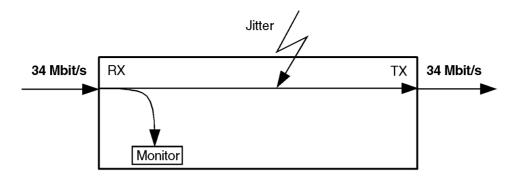
Fig. S-5 Through Mode: Adding jitter to the looped-through signal
