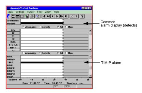
Fig. A-49 The Anomaly/Defect Analyzer window
