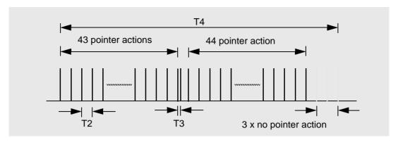
Fig. TB-9 "43-44" sequence with double pointer
