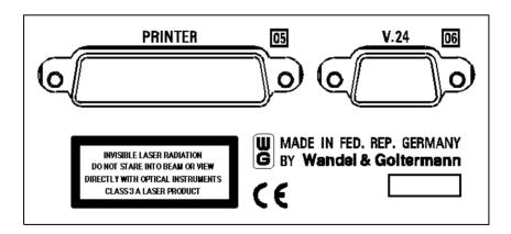
Fig. G-3 Laser safety warning label on the front panel of the ANT-20/ANT-20E
