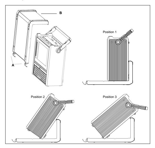
Fig. G-5 Uses of the ANT-20 protective cover
