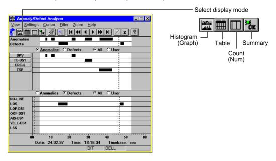
Fig. O-31 Example result display in "Anomaly/Defect Analyzer" window (View "Graph")
