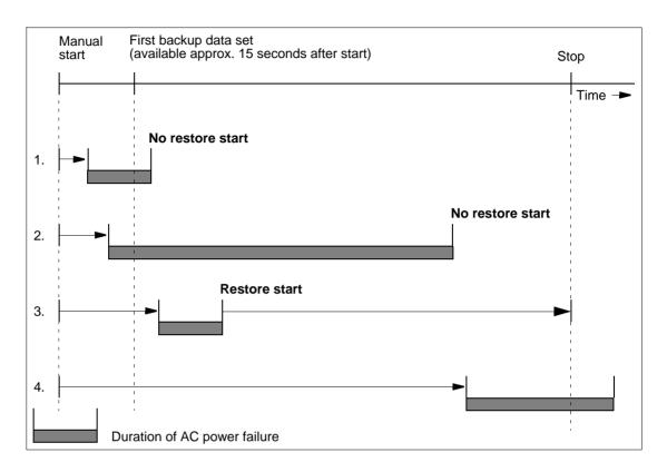
Fig. O-42 Examples of ANT-20/ANT-20E behavior in the event of an AC power failure (manually triggered measurements)
