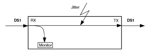
Fig. S-3 Through Mode: Adding jitter to the looped-through signal
