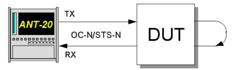
Fig. A-27 Bit error rate test setup
