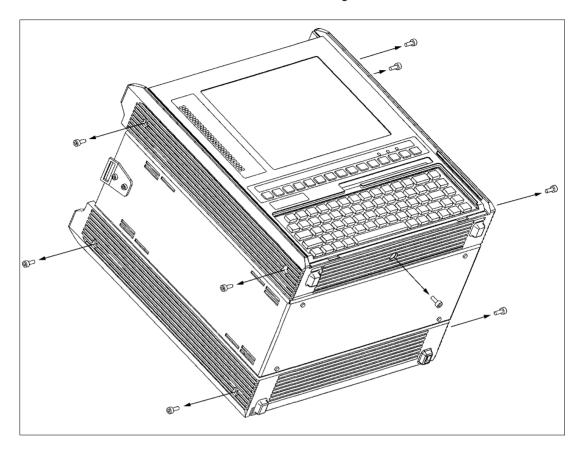
Fig. M-5 Removing the housing covers
