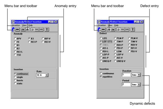
Fig. VI-8 Elements of the "Anomaly/Defect Insertion" window
