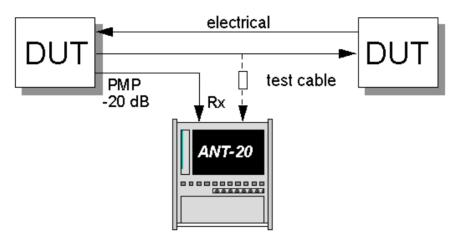
Fig. A-7 Monitoring from a protected monitoring point (PMP)
