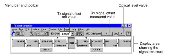
Fig. VI-1 Elements in the "Signal Structure" main window
