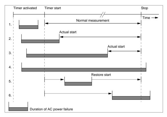
Fig. O-43 Examples of ANT-20/ANT-20E behavior in the event of an AC power failure (timer-controlled measurements)
