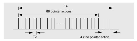
Fig. TB-10 "86-4" sequence with missing pointer
