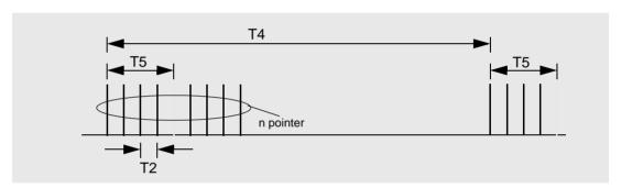
Fig. TB-7 Pointer burst with missing pointers
