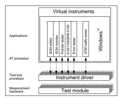
Fig. I-3 ANT-20 software architecture
