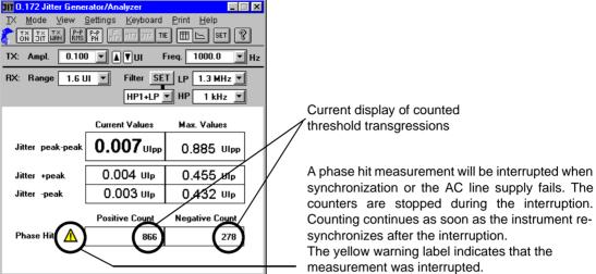
Fig. A-72 Phase hit measurement
