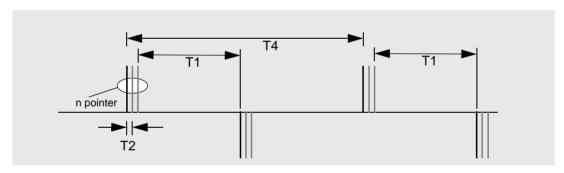
Fig. TB-4 Perodic (single/multiple) pointers with different polarity
