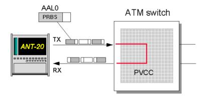
Fig. A-98 Setup for the ATM bit error rate test
