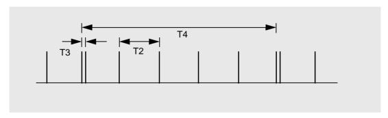
Fig. TB-5 Perodic pointers with different polarity, e.g. T4 = 5 x T2
