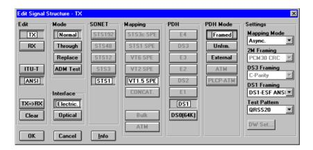
Fig. VI-2 Displaying and setting the signal structure using ANSI (Tx side) as an example
