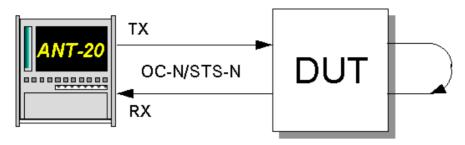
Fig. A-50 DCC/ECC bit error test setup
