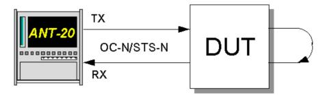
Fig. A-43 Setup for editing and analyzing the transport/path overhead
