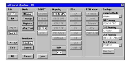
Fig. A-93 Displaying and setting the signal structure to ANSI standard
