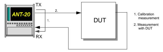
Fig. A-62 Jitter transfer function measurements setup
