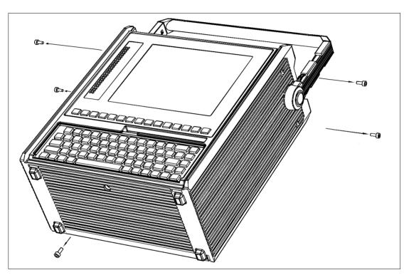
Fig. M-3 Removing the ANT-20 from its housing
