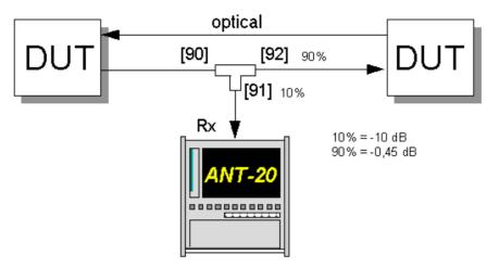
Fig. A-9 Monitoring using an optical power splitter
