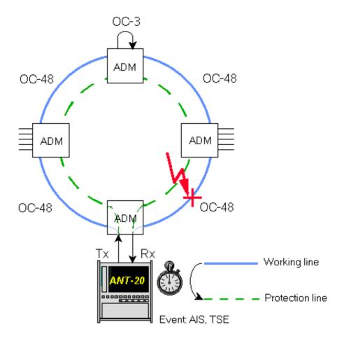
Fig. A-24 APS switching time setup
