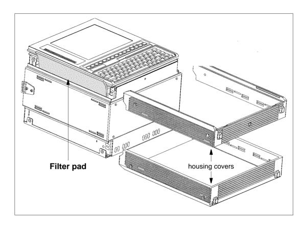
Fig. M-6 Replacing the ANT-20E filter pad
