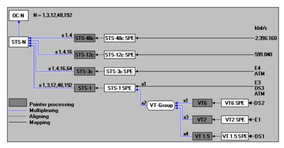
Fig. TB-1 SONET Multiplexing Structure ANSI T1.105-1995
