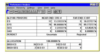
Fig. VI-40 "Performance Analysis" window showing an ITU-T M.2100 analysis
