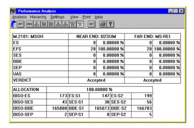
Fig. VI-41 "Performance Analysis" window showing an ITU-T M.2101 analysis
