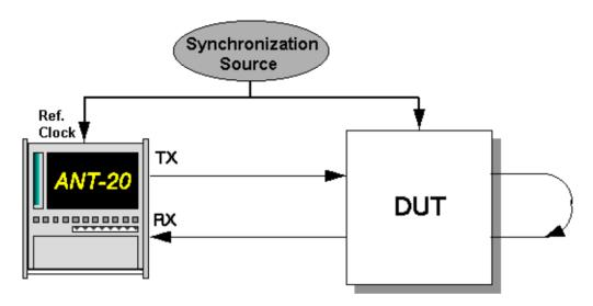
Fig. A-73 Test setup for tolerance to wander measurements
