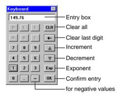
Fig. O-35 The "Keyboard" window for entering numerical parameter values
