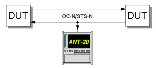
Fig. A-10 In-service monitoring setup
