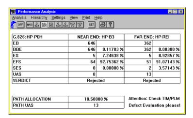
Fig. VI-37 "Performance Analysis" window showing ITU-T G.826 ISM (in-service measurement)
