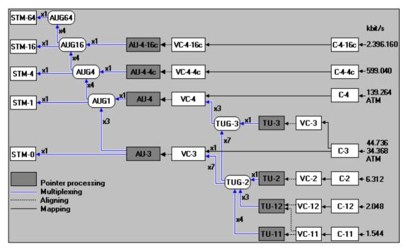
Fig. TB-2 SDH Multiplexing Structure ITU-T G.707
