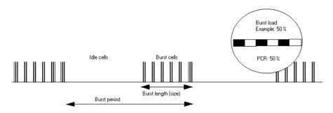
Fig. A-125 Definition of the burst period, burst length etc.
