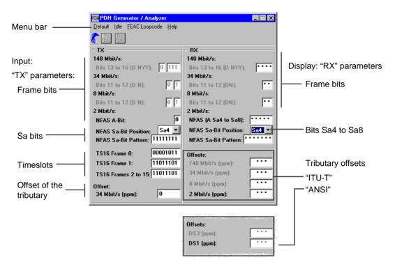
Fig. VI-31 Elements of the "PDH Generator/Analyzer" main window TX side: ITU-T signal structure, RX side: ITU-T or ANSI signal structure
