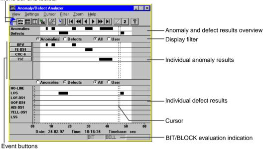
Fig. VI-9 Elements of the main window showing results as a histogram (default setting)
