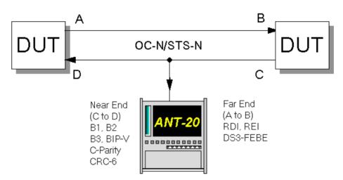
Fig. A-34 In-service monitoring setup
