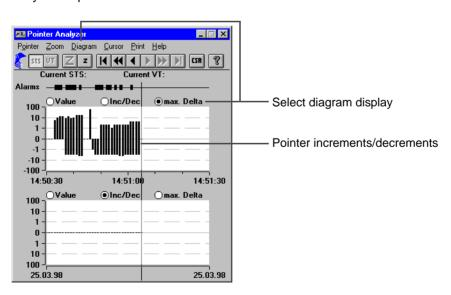
Fig. VI-28 "Pointer Analyzer" main window for Virtual Concatenation
