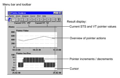
Fig. VI-27 Elements of the "Pointer Analyzer" main window
