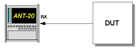
Fig. A-68 Phase hit measurement setup
