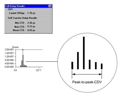
Fig. A-112 "Cell Delay Results" display window on the ATM Traffic Analyzer and definition of the peak-to-peak CDV
