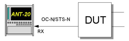
Fig. A-11 Out of service measurement setup
