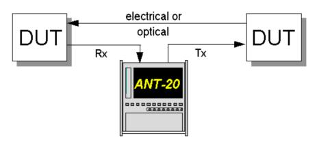
Fig. A-8 Monitoring using the ANT-20 in "Through" mode
