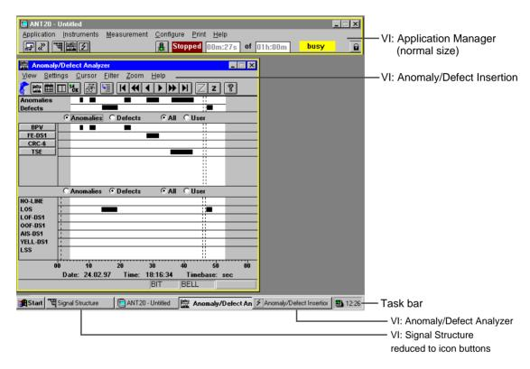
Fig. O-33 Screen display of virtual instruments
